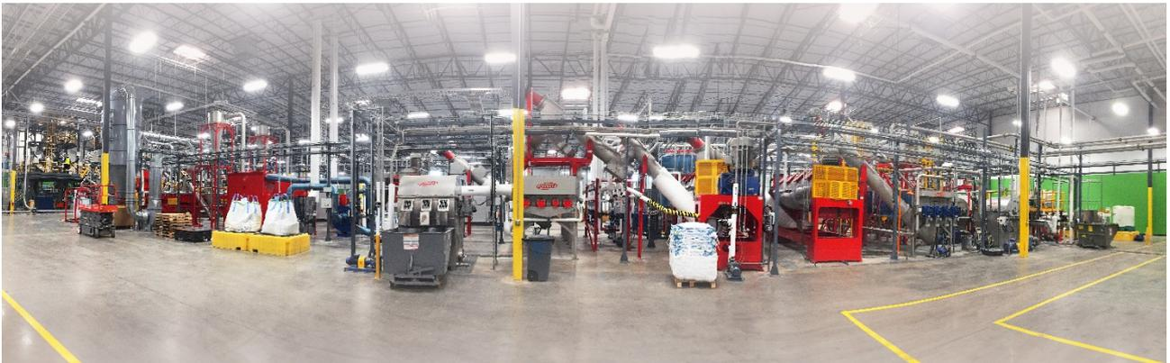
This 250.000-square-foot bottle-to-bottle PET recycling plant processes more than 100 million pounds plastic bottles annually and the AMUT washing section is capable of reaching 6 metric tons per hour (the Dallas facility will double the company’s annual capacity of food-grade PET) and permits the transformation of old plastic bottles into PET resins, flakes and pellets that can then be used to produce new beverage bottles and other sustainable products.
