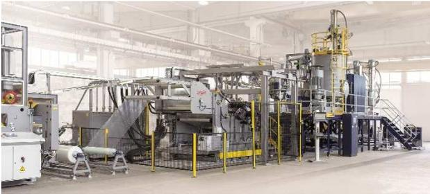
During the last months, AMUT GROUP solution to get r-PET sheet through a direct extrusion process was presented in Demo Show. This is a remarkable example of Bottle to Packaging application to meet the circular economy trend. **The line processes 100% post-consumer PET bottles flakes into certified food grade single layer foil suitable for the thermoforming phase.**
