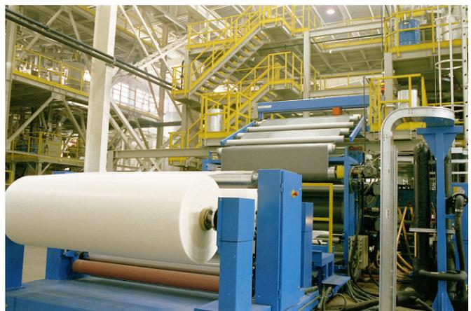
The line is also equipped with thickness gauge measuring device, high accuracy winder unit to produce jumbo and custom rolls and PC/PLC system to control all running operations of the line.
