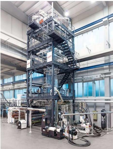
“The supply includes: three co-ex lines for blown PE shrink film, one cast line for stretch film, one slitting machine, a system for the recovery of flawed rolls, chiller, piping for water distribution plus an intensive training programme for GEPP technicians” says Riccardo Castello, AMUT DOLCI EXTRUSION Division Sales Director.
